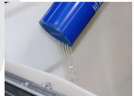
Normal Operation of the Filter: The active material allows water to pass through.
