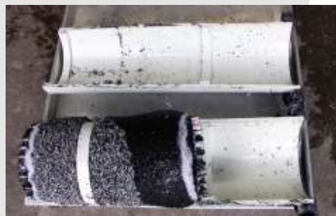
Example a PETRO PIPE saturated with hydrocarbons, cut in half, showing the active material that has formed a plug.
