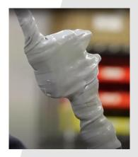
The 0.8 mm thick self-fusing silicone tape forms a custom-fit insulating barrier, delivering 15 kV phase-to-ground insulation with a single layer and up to 30 kV with a double layer. It is ideal for use on equipment with irregular or complex geometries.
